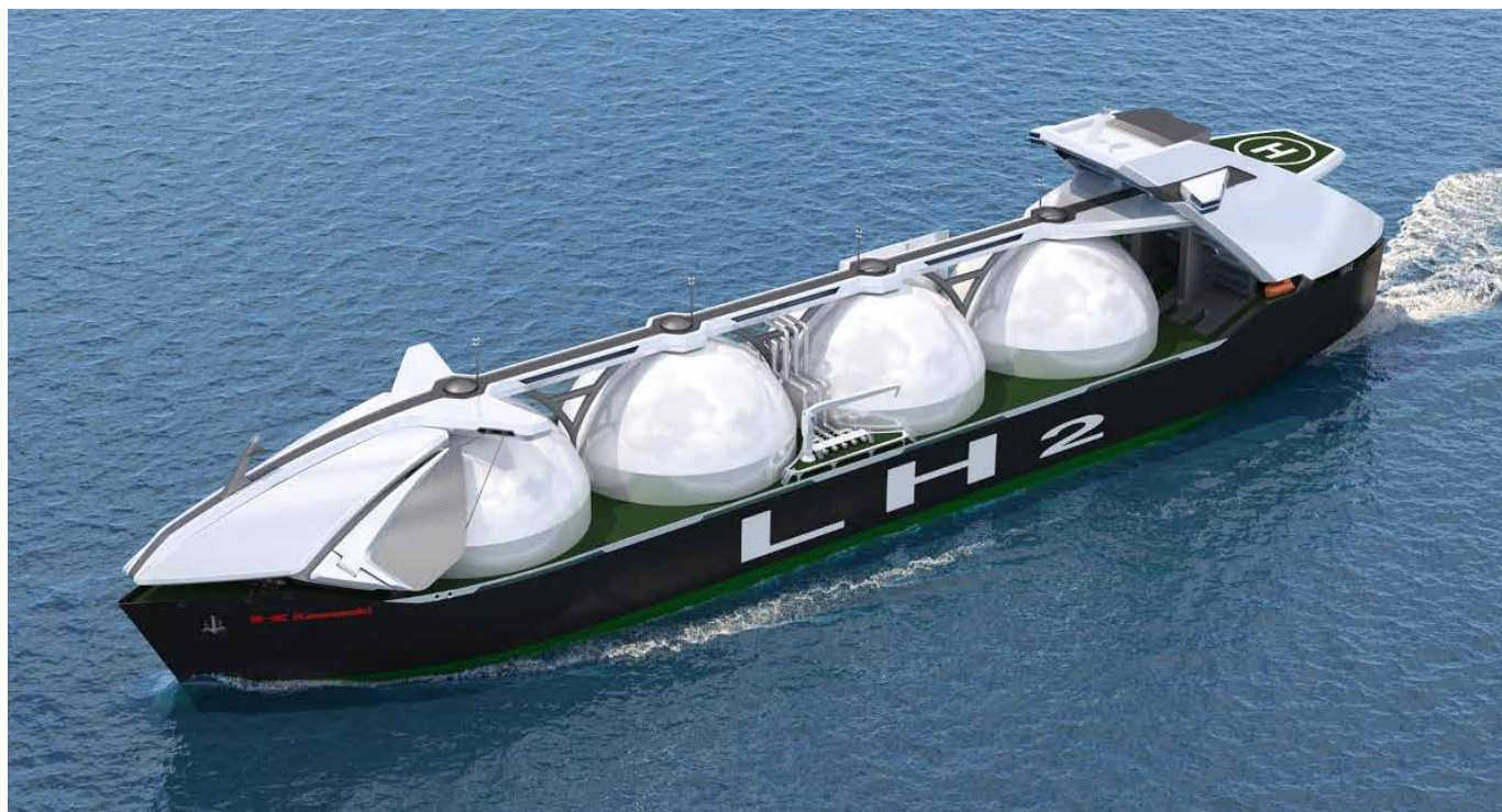
Simulated appearance of the completed 160,000 m 3 liquefied hydrogen carrier
